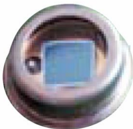
Figure 9. Series 4 PIN silicon optical sensor.
